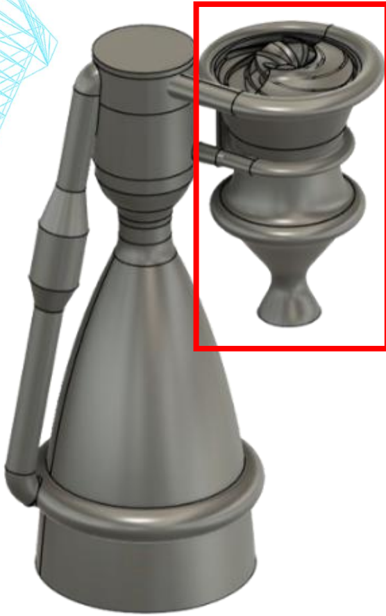
Methane/Oxygen open gas generator cycle liquid rocket engine
